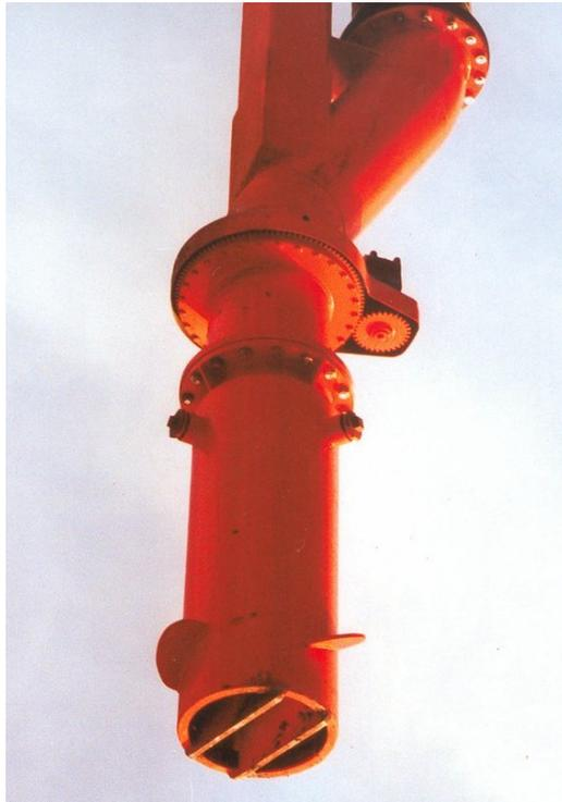
The hurricane aeration system and the rotating fluidizing nozzle improve the unloading capacity.
