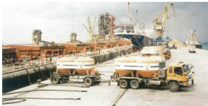
Fig. 6 In Thailand large scale cement exports are realised with little more than the use of bulk trucks. Loading rates of 10.000 tons per day have been achieved this way.
