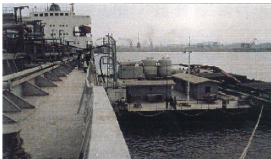
Fig. 5 Cement exports by Lafarge out of Romania. In Constanza a floating facility transfers cement from inland barges directly into large bulk carriers
