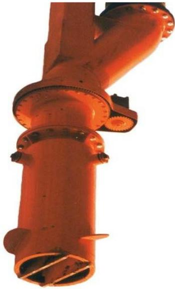
operated, low speed cutting head, which loosens and fluidises the (packed) material. By proper fluidising of the cement, before it is sucked into the system, the capacity of the unit increases. But the main advantage of the fluidisation of the cement is that the stresses on the arm are reduced significant. And while the stresses are reduced, the lifetime of the arm is much longer.
