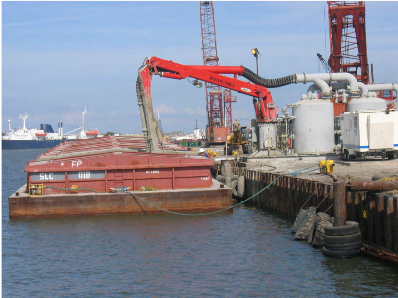
Barge unloading by 180 tph pneumatic unloader
