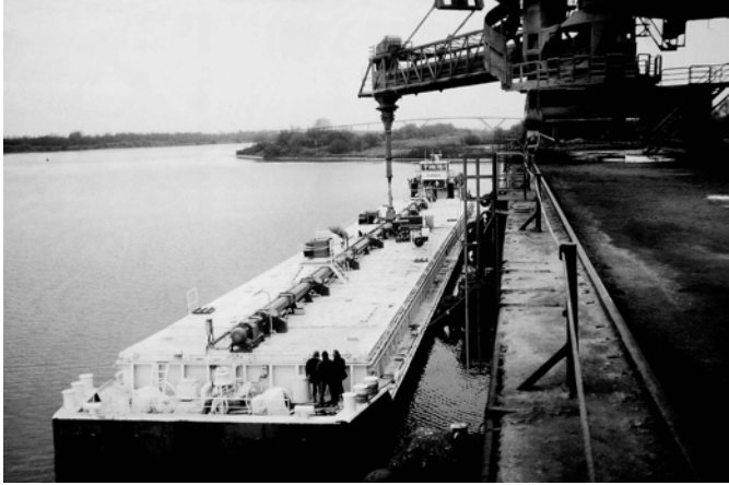
(Fig. 5 IBAU screw conveyor for loading/unloading)
