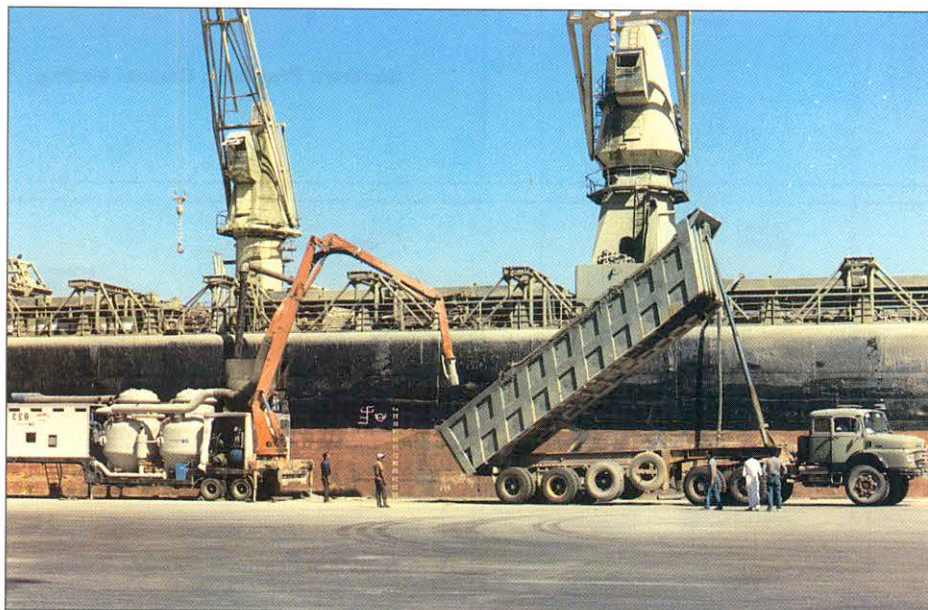
Jordan Cement, Port of Aquaba. A Kovako type road mobile unloader conveys cement from large tipper trucks directly into a large bulk carrier.
