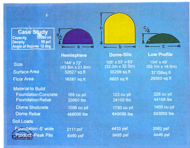
Figure 5. Comparison of different dome configurations (courtesy of Dome Technology).
