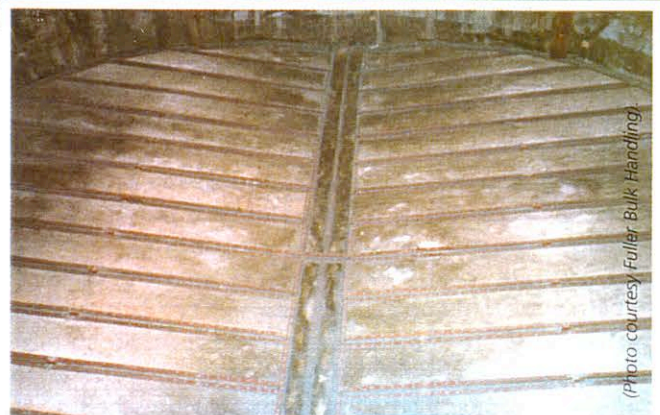
Figure 1. Full fluidised floor with side outlet. The inclined bottom slopes both to the centreline and to one side of the dome where the outlets are located. The sections of the floor are clearly visible. (Photo courtesy Fuller Bulk Handling).
