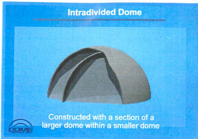
Figure 6. Single dome suitable for multiple products storage (courtesy Dome Technology).
