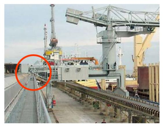
• Fixed position of shore transfer system makes barge mounting impractical
