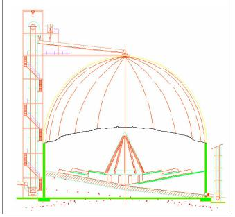
Cement within the silo is guided into the pressure relief chamber from the sections of the outer rings via small discharge tunnels which pass beneath the inner floor ring area. From the inner aeration ring cement flows directly into the relief chamber via radial fluidslides. This design
