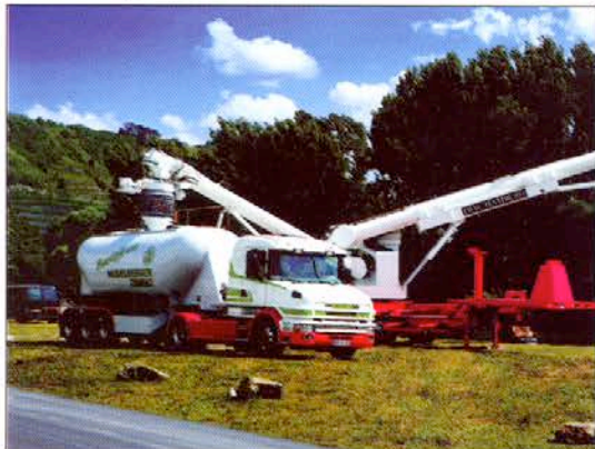
Roadmobile unloaders can be moved over the road with little or no disassembly
