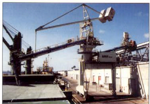
For large import terminals with a high annual throughput and an infrastructure with existing rails, the railmounted mechanical unloader (pictured above and below) is almost a natural selection
