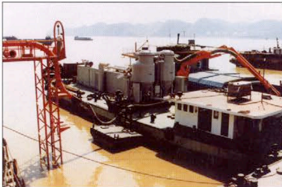
Barge-mounted systems can easily cope with large differences in waterlevel. Due to the simple rubberhose connection with the shore, pneumatic systems are attractive for such applications
