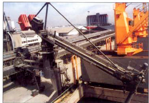
For large import terminals with a high annual throughput and an infrastructure with existing rails, the railmounted mechanical unloader (pictured above and below) is almost a natural selection
